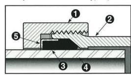
Threaded end-nuts screw onto the threaded body
